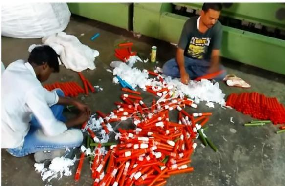
Fig.4.1 Labour removes waste yarn from bobbins
