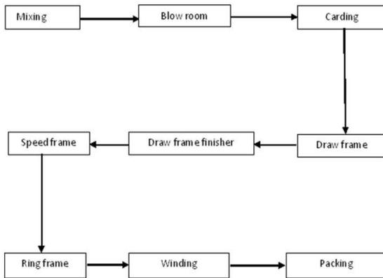
Fig.2 Yarn manufacturing process
