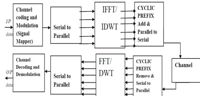
Figure 1: Block diagram of a OFDM system.
