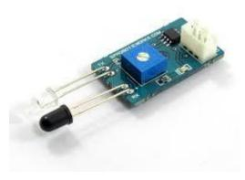
All objects which have a temperature greater than absolute zero (0 Kelvin) posses thermal energy and are sources of infrared radiation as a result. Infrared sensors typically use infrared lasers and LEDs with specific infrared wavelengths as source.
