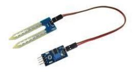
Soil moisture sensors measure the volumetric water content in soil. Since the direct gravimetric measurement of free soil moisture requires removing, drying, and weighting of a sample, soil moisture sensors measure the volumetric water content indirectly by using some other property of the soil, such as electrical resistence, dielectric constant, or interaction with neutrons, as a proxy for the moisture content
