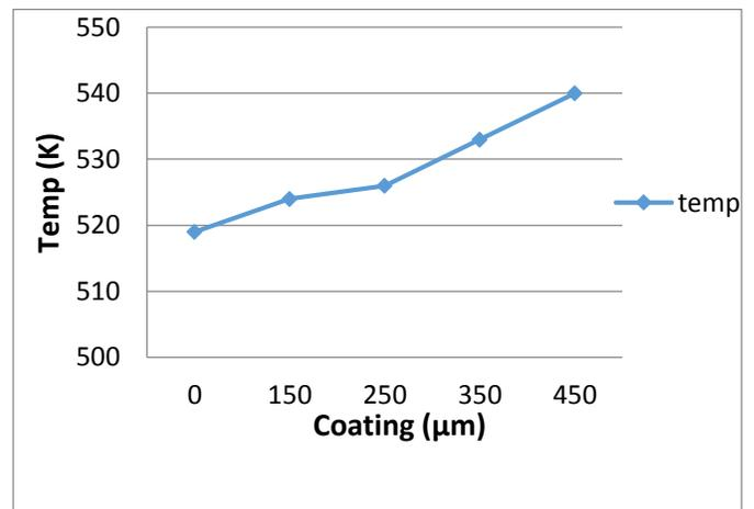
Fig. 5. Graph representing change in the variation of temperature at the top surface of piston with increasing thickness of coating
