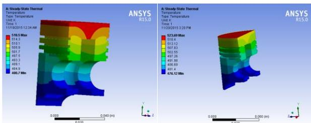
Fig.4 (a) Temperature distribution for uncoated piston Fig. 4(b) Temperature distribution for 150 micron coated piston.
