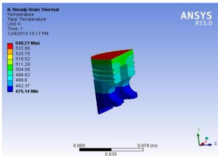
Fig. 4(e) Temperature distribution for 450 micron coated piston.
