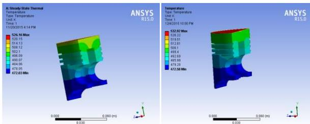
Fig 4(c) Temperature distribution for 250 micron coated piston. Fig.4 (d) Temperature distribution for 350 micron coated piston.
