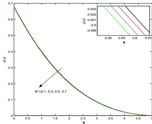
Fig.21. Effect of temperature dependent heat source/sink parameter  $B^*$  on  $\phi(\eta)$
