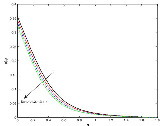
Fig.7 Effect of stretching parameter  $s$  on  $\theta(\eta)$
