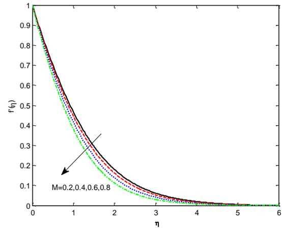
Fig.5. Effect of Magnetic field parameter  $M$  on  $f'(\eta)$
