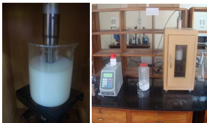
Figure 2: Photographs of Nano Fluid: (a) Mixture of TiO 2 and Base Fluid in Conical Chamber, (b) Ultrasonic Vibrator Experiments
