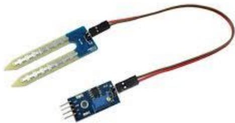
Soil moisture sensors measure the volumetric water content in soil. Since the direct gravimetric measurement of free soil moisture requires removing, drying, and weighting of a sample, soil moisture sensors measure the volumetric water content indirectly by using some other property of the soil, such as electrical resistance, dielectric constant, or interaction with neutrons, as a proxy for the moisture content
